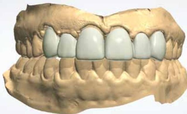
**(4) Restoration Design** – Image shows two 3-unit High Translucency Full Zirconia bridges #6-8 and #9-11 designed in the 3Shape software.
