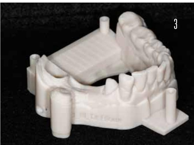
**(3) Printed Model -** Image shows the model after being printed in the Carbon M1 Printer and post processed. Models are printed with removable dies which provide highly accurate margin replication while maintaining the soft tissue captured in the digital impression. This allows the designers to follow the tissue contour and create a very natural (not bulky) emergence profile for the restorations.
