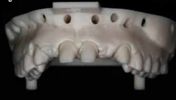
**(3) Printed Model** – Image shows the model after being printed in the Carbon M1 Printer and post processed. The holes in the base of the model allow it to be removed from the printer build platform quickly and easily.
