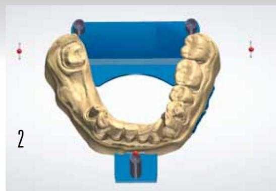
**(2) Model Design -** Image shows the model being built in the 3Shape Model Builder software.
